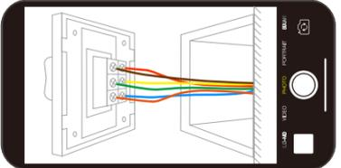
• Follow the wiring diagram to connect the switch wires to the wires in the wall box with the wire conductors.
